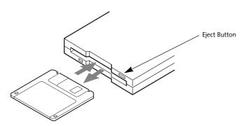
Figure 4-4.Loading/Ejecting a 3.5" Floppy Disk
